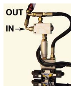
Elettroil connection to quick-fit couplings of the tractor
